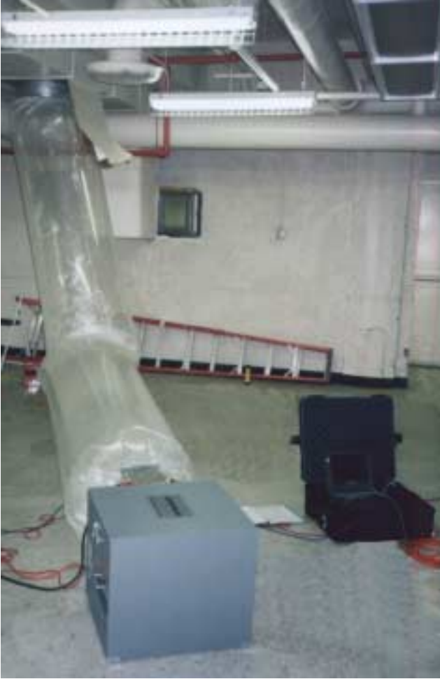
Figure 4. Aerosol injection machine connected to Building LS-2 via 0.65 m (25.5 inch) diameter lay-flat polyethylene tubing
